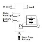
Input: Single-phase 115 - 277 Vac Output Load: power supply 24 Vdc; 3 A Output Battery: charging 24 Vdc; 3 A
